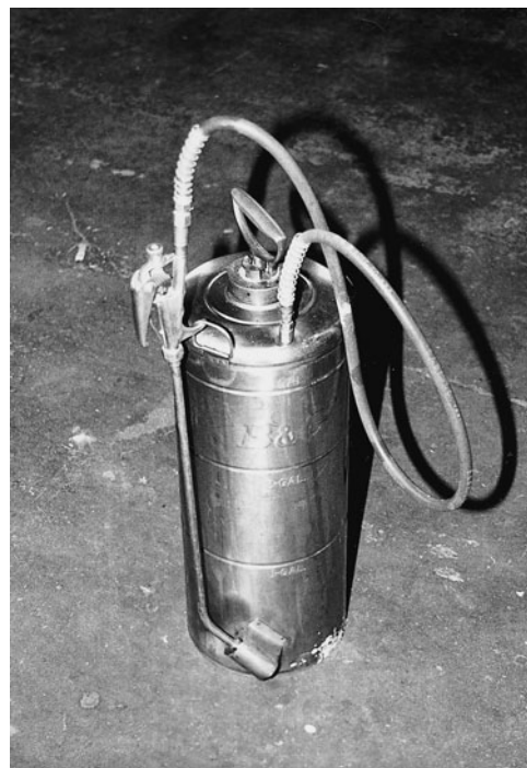
FIGURE 8-8 Compressed-air tank sprayer. (Source: George Acquah)
