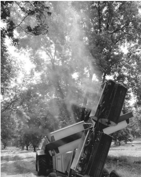
FIGURE 8–9 A tractor-mounted sprayer for trees. (Source: USDA)
