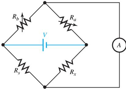
**Figure 1.4.2** Basic Wheatstone bridge circuit for resistance measurement.
