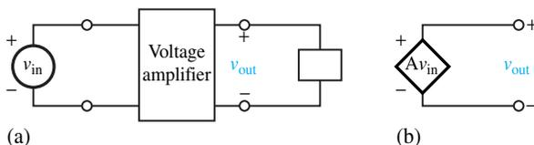
**Figure 1.1.7** Voltage amplifier and its controlled-source model.
