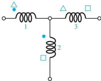
**Figure 1.2.11** Polarity markings for complicated magnetic coupling situations.
