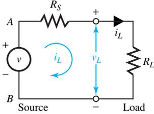
**Figure 1.2.3** Power transfer between source and load. *Note:*  $R_L = 0$  implies short circuit;  $v_L = 0$  and  $i_L = \frac{v}{R_S}$  and  $R_L \rightarrow \bullet$  implies open circuit;  $i_L = 0$  and  $v_L = v$ .
