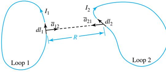
**Figure 1.1.2** Illustration of Ampere’s law (of force).
