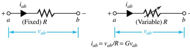
**Figure 1.2.1** Circuit symbols of fixed and variable resistors and illustration of Ohm's law.
