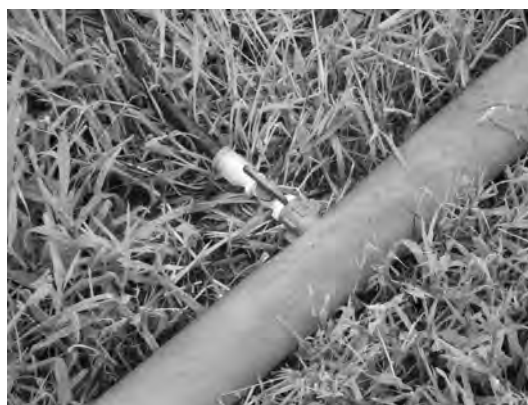
Fig. 7.4. Trickle irrigation showing lay-flat supply hose connected to trickle tape via an adjustable valve for regulating water supply.
